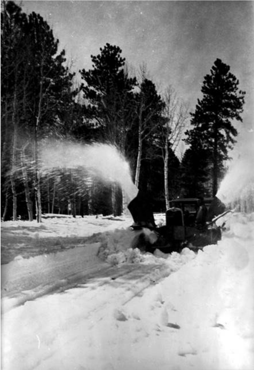
#15543: SNOW BLOWER DEVELOPED BY SOUTH RIM MAINTENANCE, BEING USED TO OPEN THE NORTH RIM ROAD, CIRCA 1937. PHOTO BY WARREN HAMILTON.
